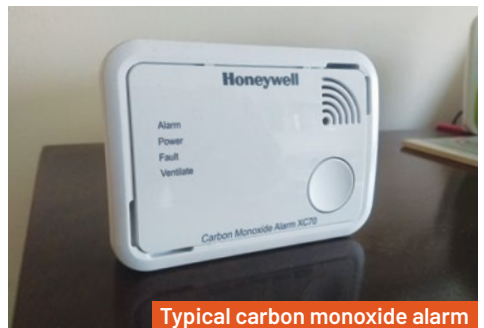
Typical carbon monoxide alarm
