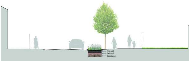
Section A-A' Existing pavement | Permeable paving rainwater collection system | Proposed rain garden | Existing pavement | St Mary's C of E Primary School
