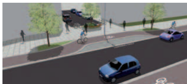
Inset loading bay in junction of closed road with segregated cycle track
