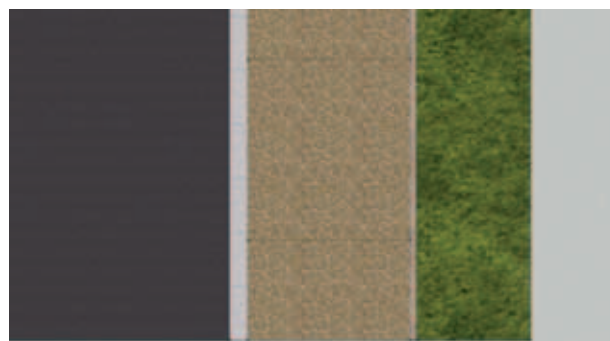
Good reinstatement over full section of path
