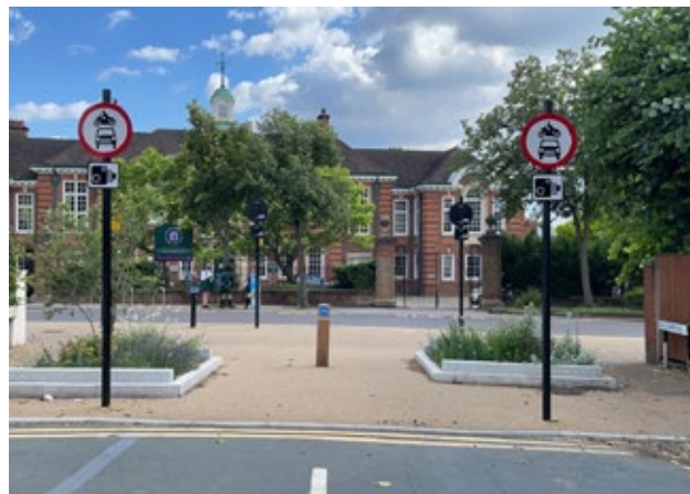
Modal filter at junction of Rectory Road and Church Hill
