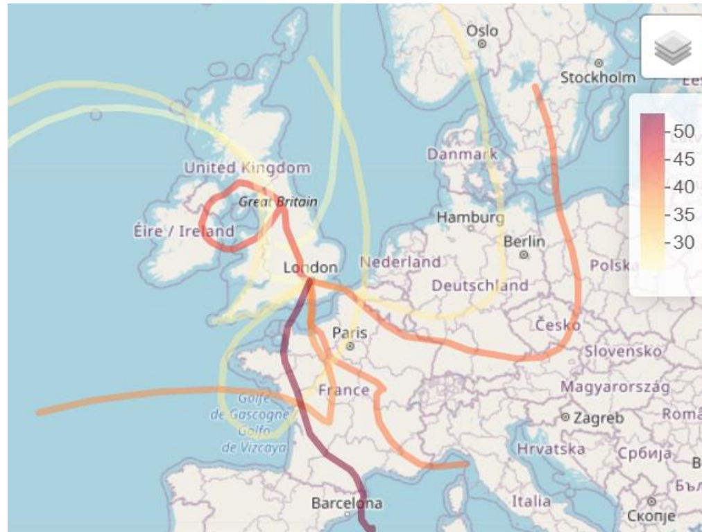
Figure 1.4 The back trajectory plot shows data from the HYSPLIT model (NOAA HYSPLIT 3) run in analysis mode. This shows the air mass back trajectories associated with top ten most polluted days in March (highest monthly mean for PM 2.5 ); these provide information on the trajectory direction associated with the top 10 measured concentrations.
