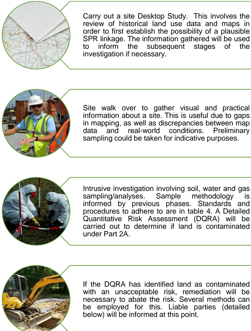
Figure 3: The Detailed Inspection and Investigation Process
