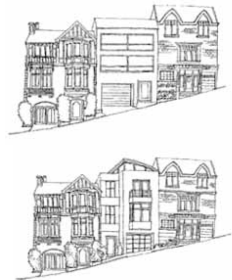
Contemporary responses to infill development taken from Bexley's residential design guide. The top image does not reference cues from its context and works less well than the lower example
